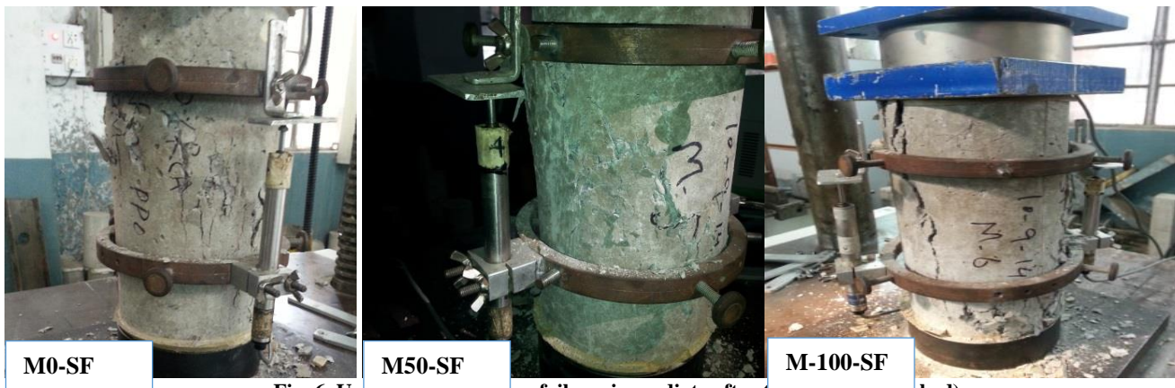
Fig. 6. Uniaxial compression failure, immediate after testing (Unsturbed)
